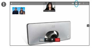
With self-view activated (see previous page) or a layout involving a picture-in-picture, navigate to **Layout** (Interpret in the upper right corner and press **OK**. The **Layout** icon will appear only when relevant.
